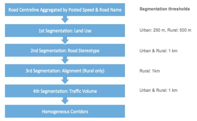
Figure 2. Corridor Aggregation Process and Segmentation Thresholds
